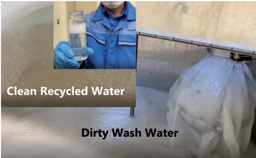
plate processing, with only the remaining 25%, in the form of a slurry or sludge, to be disposed of. Forty percent of the additive used in the water wash remains in the filtered water, reducing the amount of additive required for processing subsequent plates.
