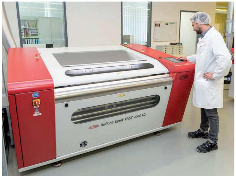
DuPont Cyrel solvent-free thermal plate-manufacturing system FAST 2000 TD
