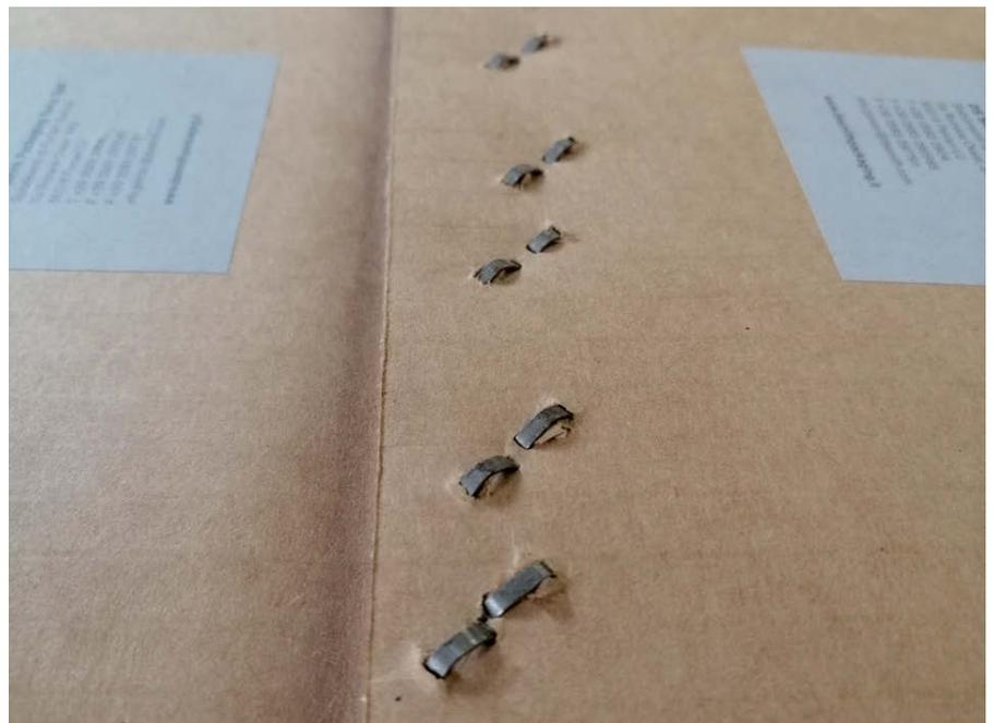
Two samples of 16mm thick TRI-WALL cardboard stitched by the XC32.1
