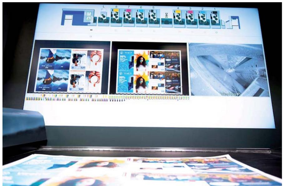
Quality sheet for sheet: QualiTronic PDFCheck combines inline colour measurement, sheet inspection and comparison with the pre-press PDF
